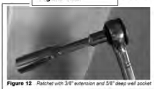
Figure 12 Ratchet with 3" extension and 5/8" deep well socket
