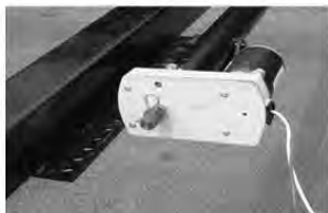
Fig. 3-Hex Head Crank Extension
