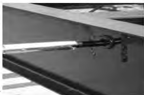
Fig. 2-Through Frame Crank Extension w/Pin
