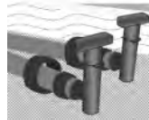
Low Point Drains
