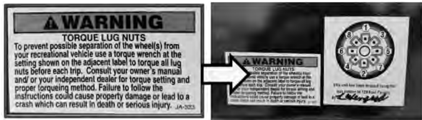
Lug nut torque pattern and warning label
