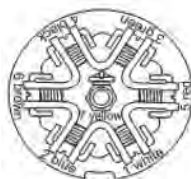
7-way trailer plug car end, rear view
