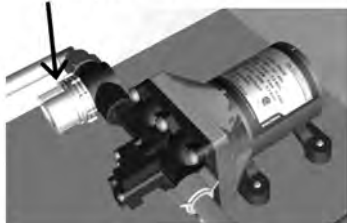
Water pump strainer
