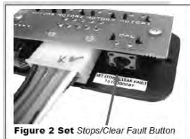
Figure 2 Set Stops/Clear Fault Button
